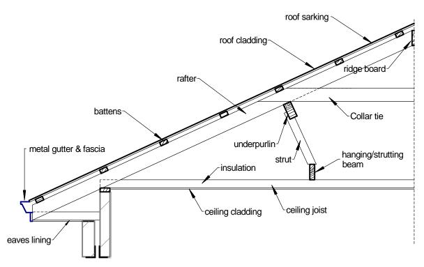
If you select the roof as element the largest part will be timber with some other materials that's shown in the above sketch. Specify the timber that you will use (stress grade, sizes etc.) and name a supplier for the timber and the accessories (nails, bolts, galvanised straps & brackets etc.)
