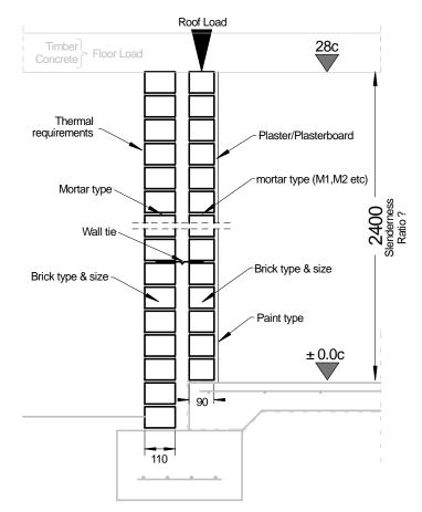
Address the issues similar requirements as for the Internal wall Element
